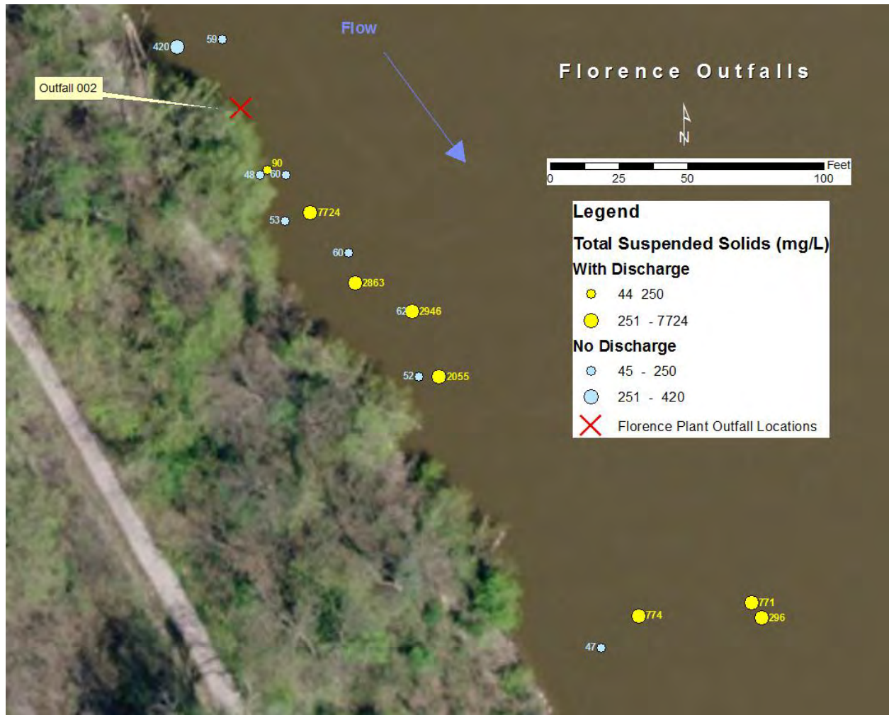
Figure 8. Florence Outfall 002 Total Suspended Solids Measurements.
