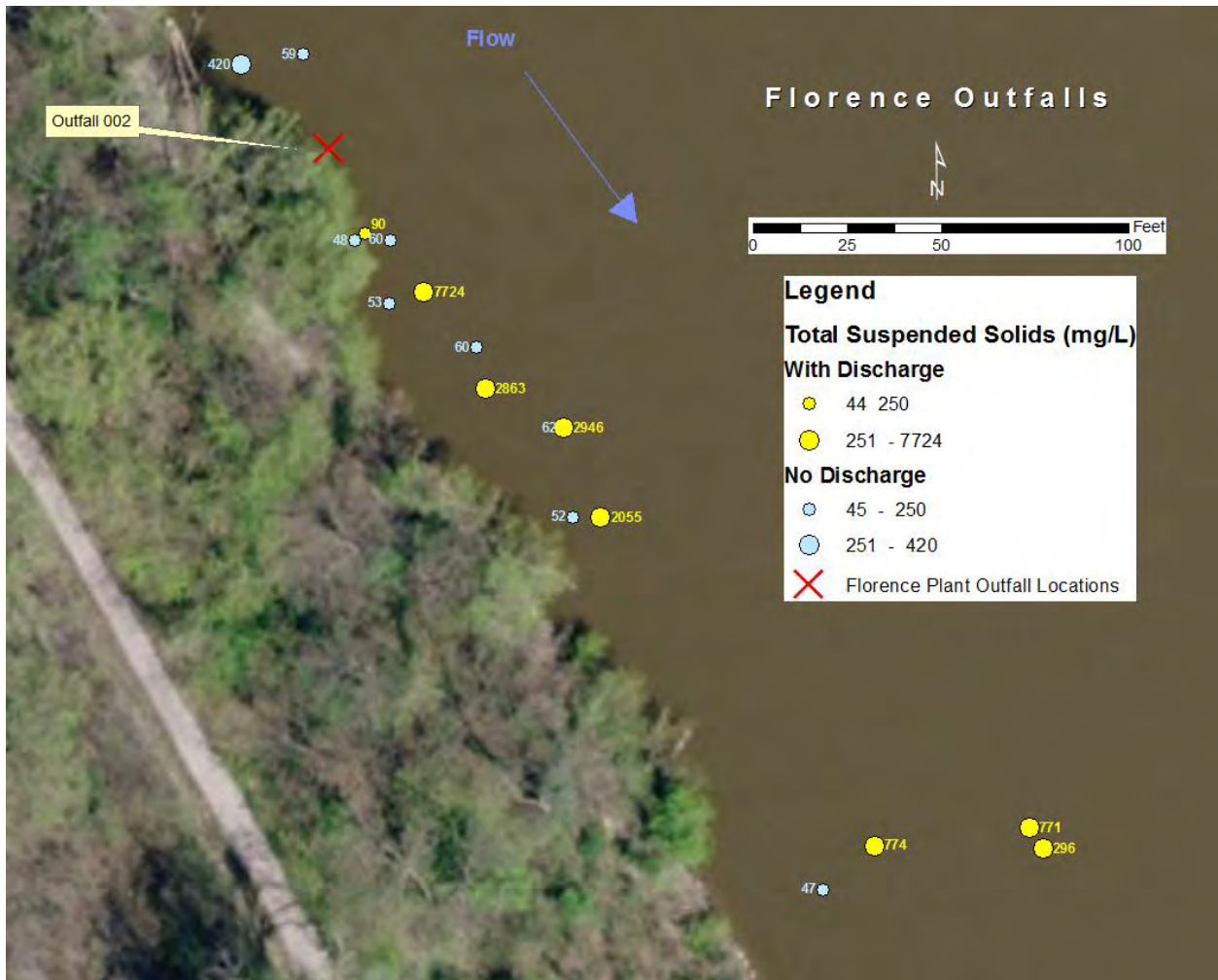
Figure 13. TSS levels measured at Outfall 002 with and without discharge
