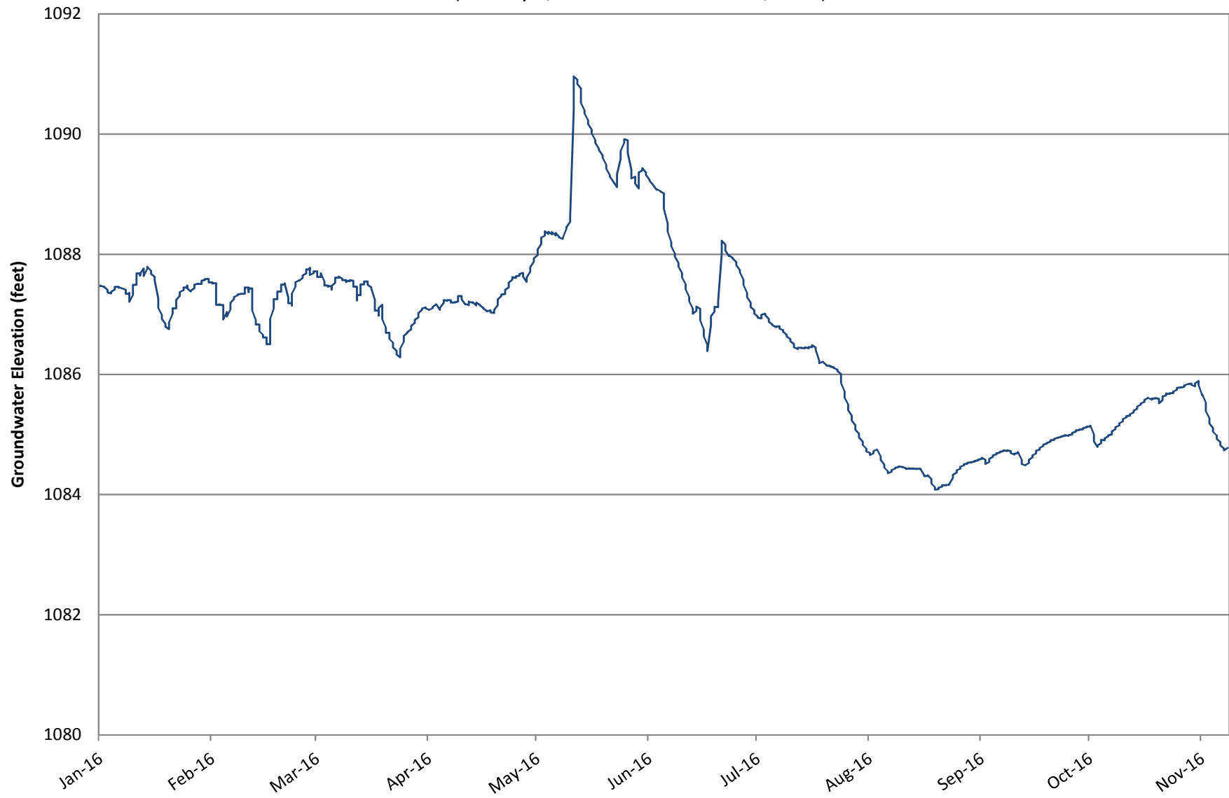
Figure 10 Monitoring Well Readings for MW 94-04 in Saunders County (January 1, 2016 thru November 8, 2016)
