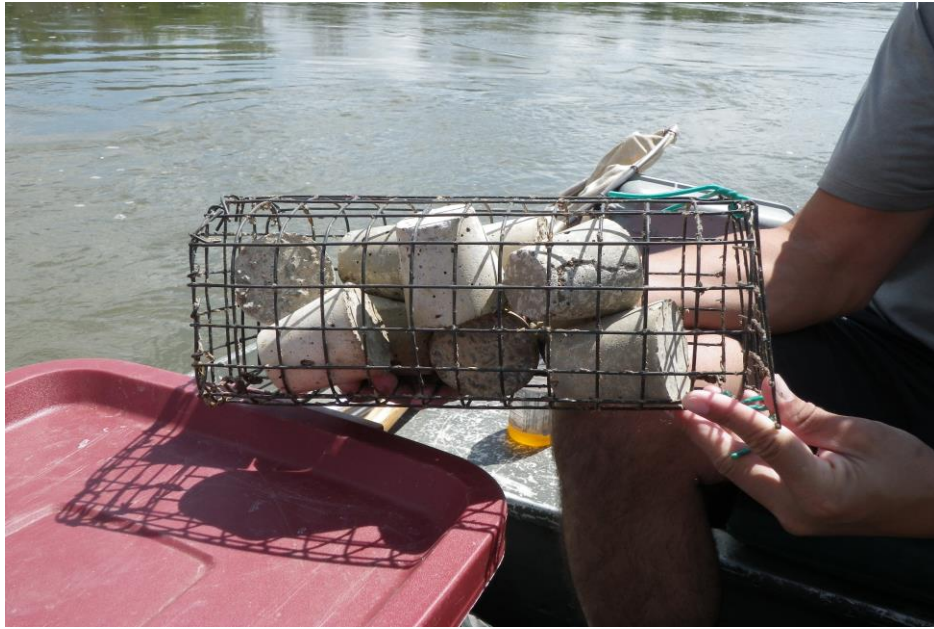
Photo 1. Artificial substrate sampler prior to placement, June 25, 2012.
