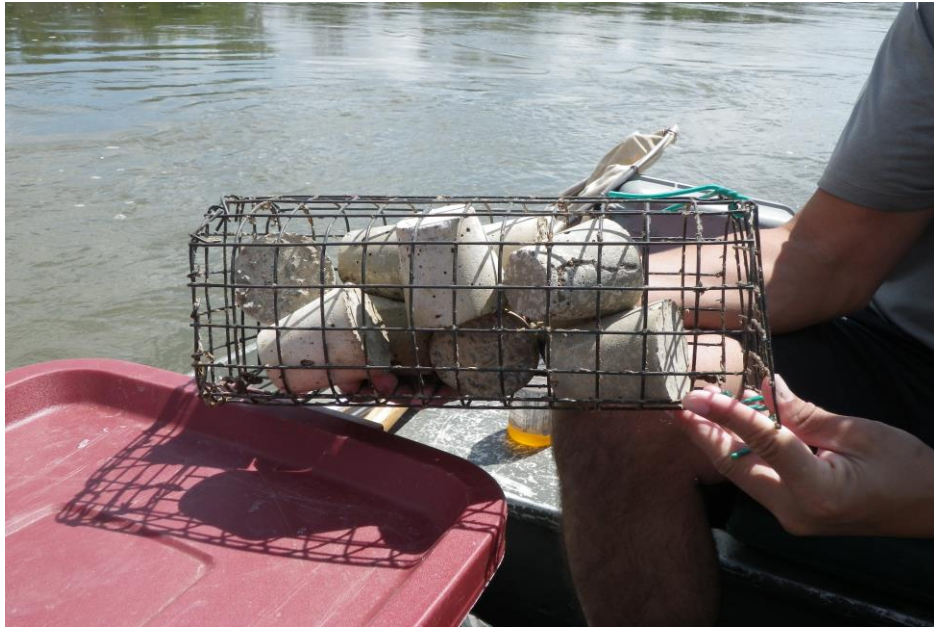
Photo 1. Artificial substrate sampler prior to placement, June 25, 2012.
