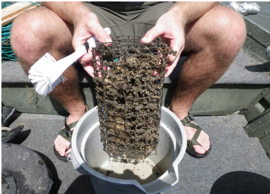
Photo 2. Artificial substrate sampler approximately 6 weeks after placement, August 13, 2012.
