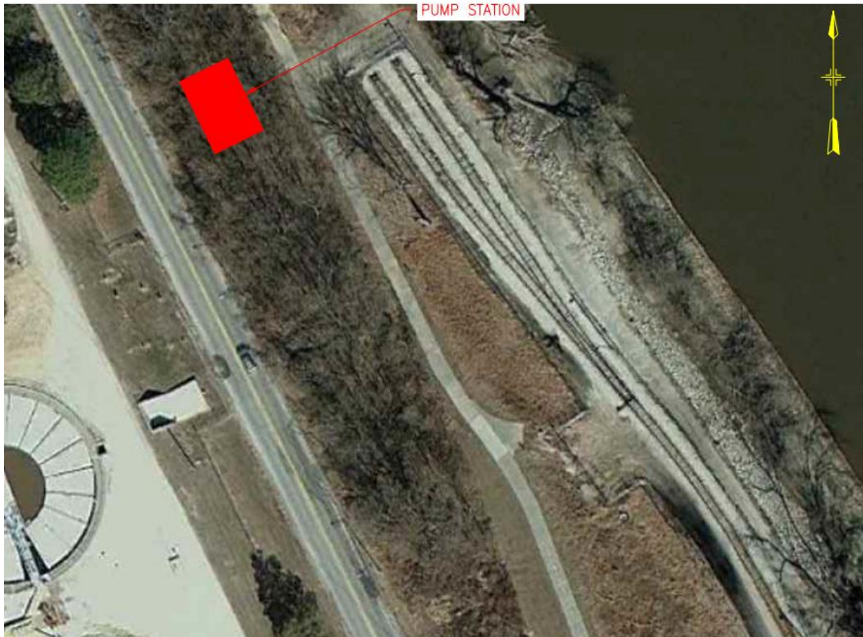
Figure 13. Location of potential clarifier blowdown pump station at Florence PWTP
