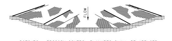
DITCHES - EROSION CONTROL BLANKETS SHALL BE APPLIED PARALLEL TO THE FLOW WITHIN THE DITCH. USE CHECK SLOTS AS REQUIRED. AVOID JOINING MATERIAL IN THE MIDDLE OF THE DITCH IF AT ALL POSSIBLE.
