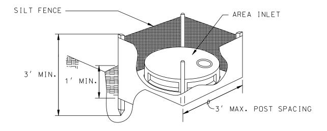
**FIGURE 3.** Typical area inlet silt fence barrier installation detail.
