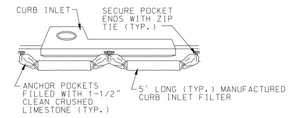
FIGURE 2. Typical curb inlet filter installation detail.
