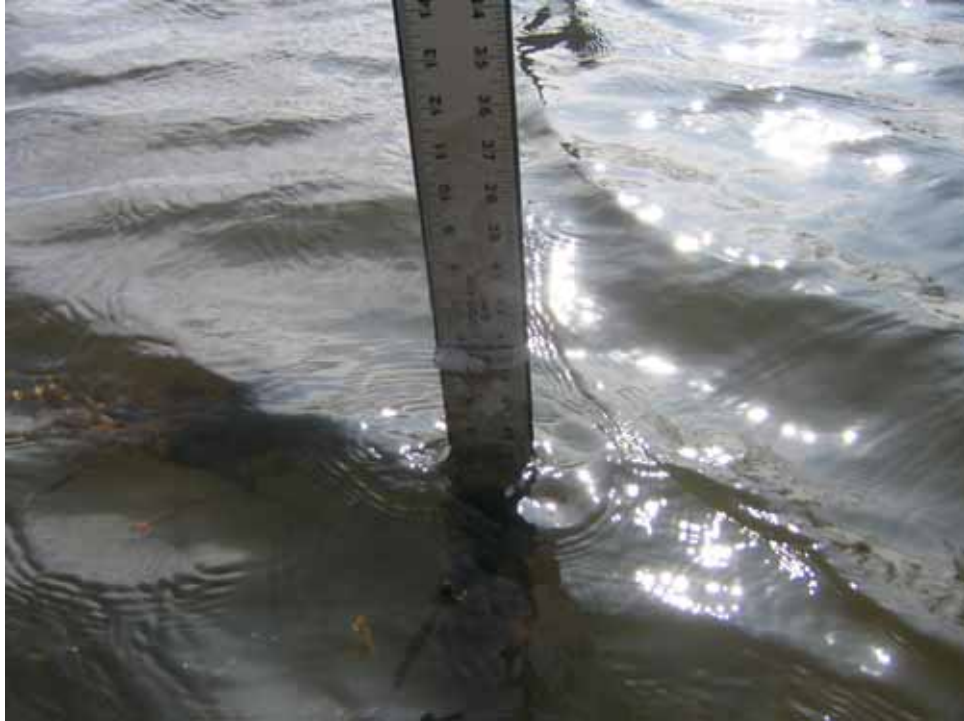
Photograph 1: View of DG-13 high water staff gauge , April 5, 2006.
