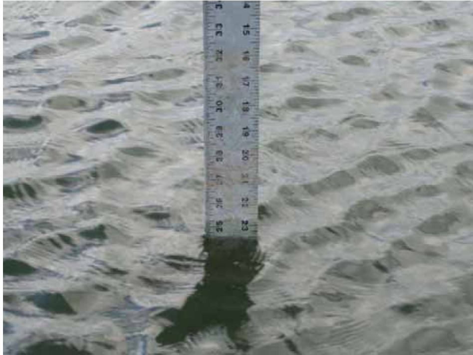
Photograph 9: View of DG-04B, staff gauge, September 19, 2006.
