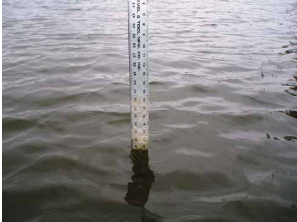
Photograph 13: View of DG-04B, staff gauge, October 16, 2006.
